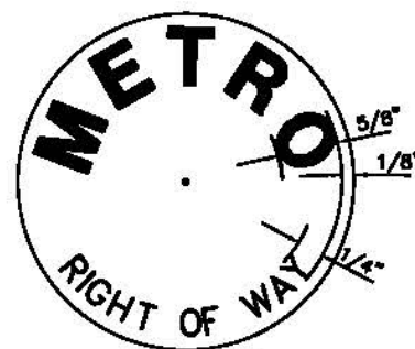
DETAIL 'I' TYPE II, III, IV, VII, VIII - TYPICAL RIGHT OF WAY CAP INSCRIPTION LAYOUT
