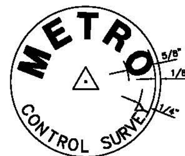
DETAIL 'J' TYPE II, III, IV, VII, VIII - TYPICAL CONTROL SURVEY CAP INSCRIPTION LAYOUT
