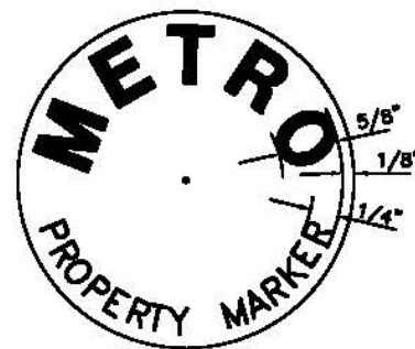
DETAIL 'H' TYPE II, III, IV, VII, VIII - TYPICAL BOUNDARY MONUMENT CAP INSCRIPTION LAYOUT
