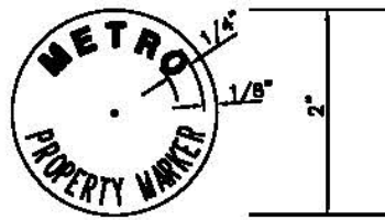
DETAIL 'C' TYPE I, VI - TYPICAL REBAR CAP BOUNDARY MONUMENT CAP INSCRIPTION LAYOUT
